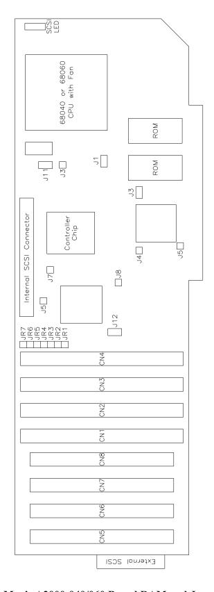
Figure 3.6: TekMagic A2000-040/060 Board RAM and Jumper Settings
