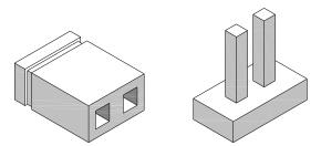
Figure 3.1: Jumper block and pins
